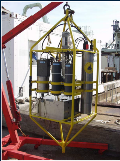
Robotic Analyzer for the TCO 2 System (RATS). Sayles et al (2009, DSR), recent pH addition by W. Martin and D. McCorkle.
