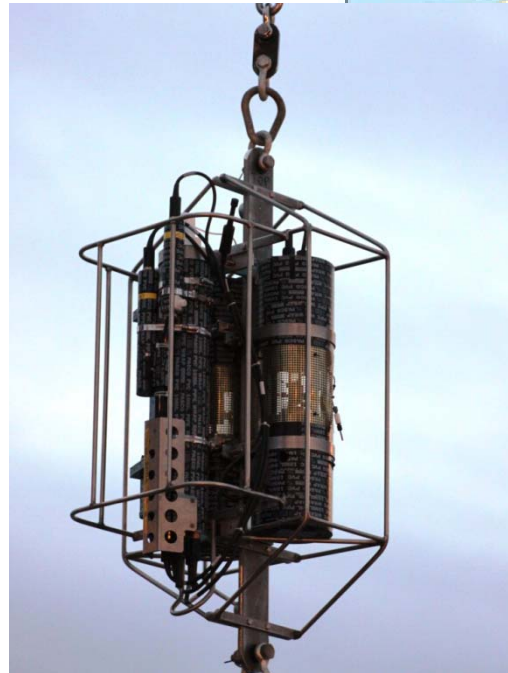
Bottom package with SAMI pH and p\text{CO}_2 , ISUS nitrate, and SBE 16+
