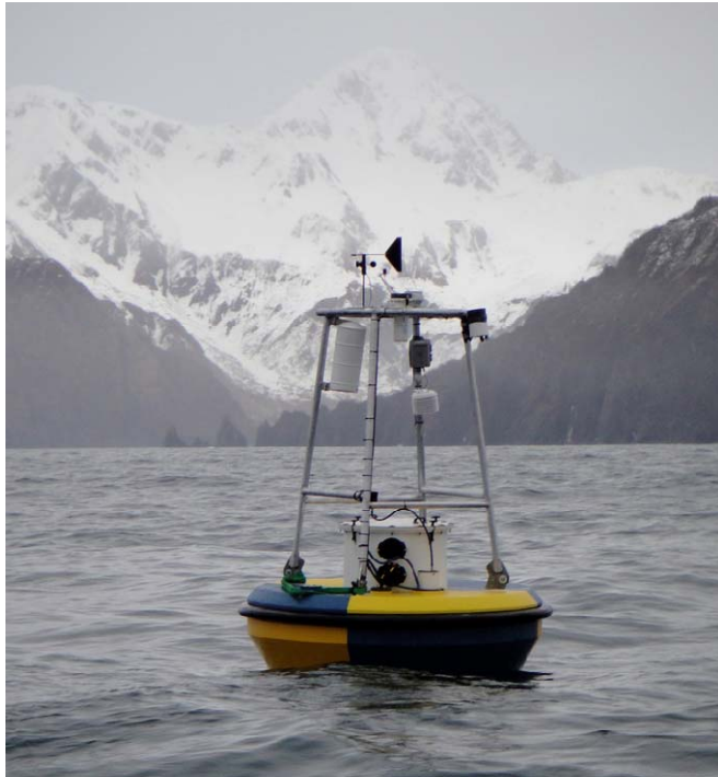
Surface buoy with MAP CO 2 System, SAMI pH, ISUS nitrate, and SBE 16+
