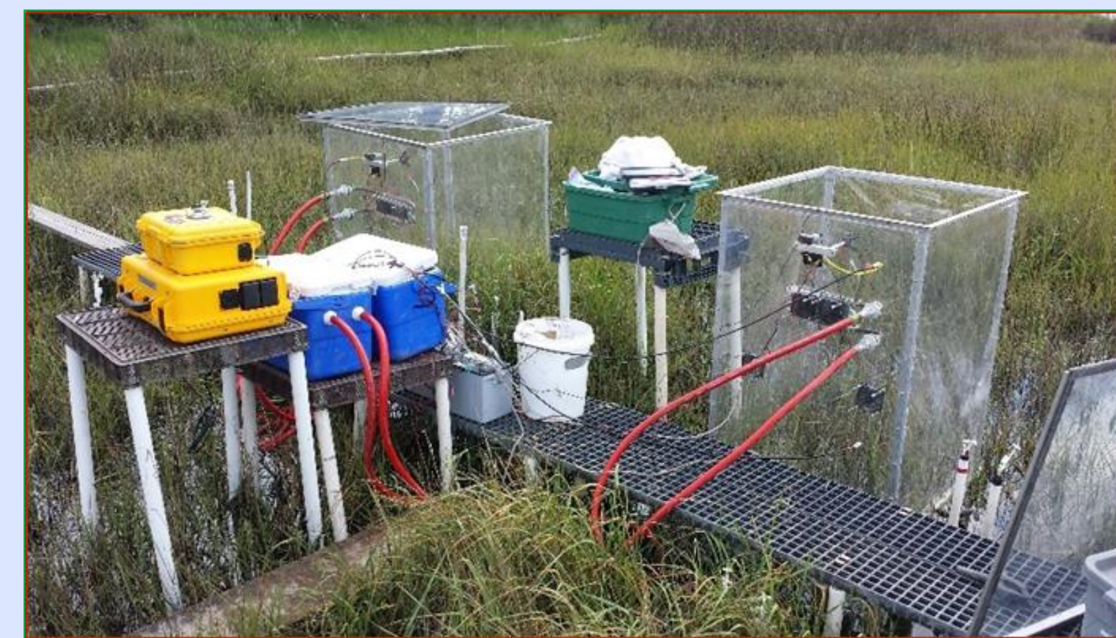
Figure 5: Chamber system for in situ CO_2 flux analysis
