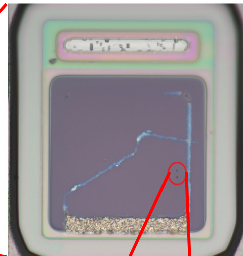
Figure 14. Optical image of the capacitor with much of the polysilicon chemically removed (some residual remains). The capacitor dielectric is exposed. The red oval indicates two pinholes in the dielectric layer.
