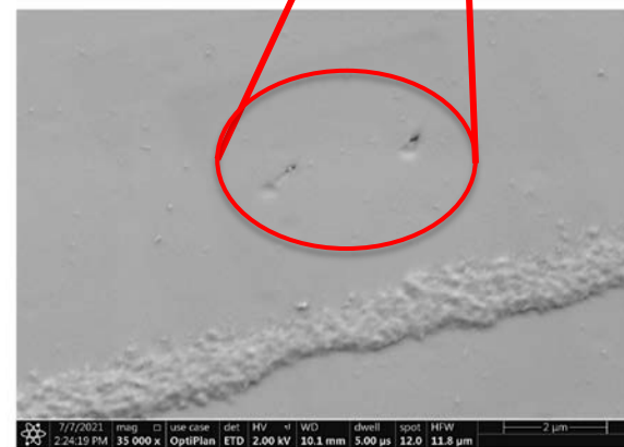
Figure 17. Tilted and rotated SEM image of the pinholes in the dielectric layer.
