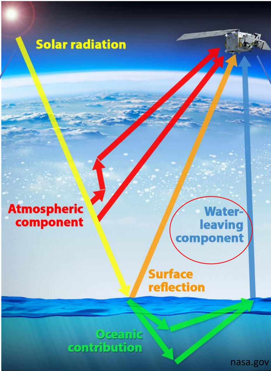
$$\text{Light reaching the satellite} = \text{Light in the atmosphere} + \text{Light reflected off the ocean} + \text{Water-leaving component of light}$$
